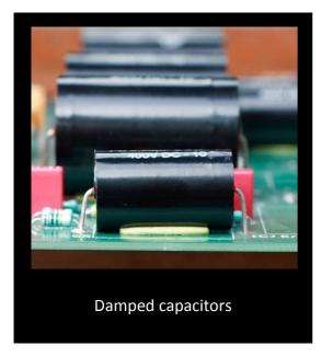
Anti vibratory material fixed on the top chassis box.
